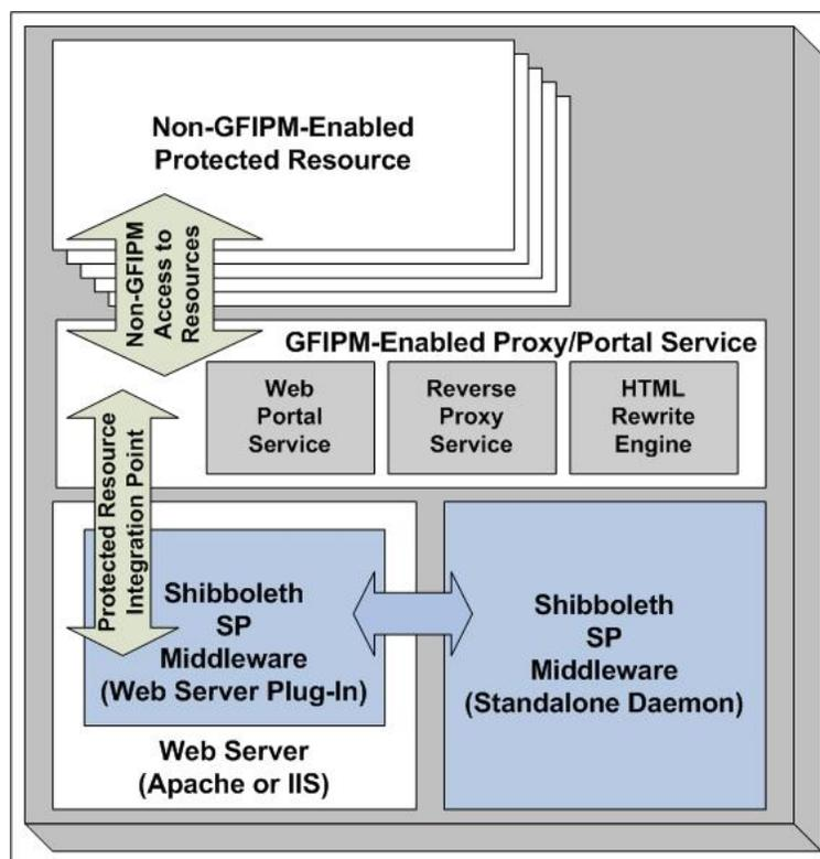
Figure 5: GFIPM Service Provider (SP) Structure with a GFIPM-Enabled Portal/Proxy Service
