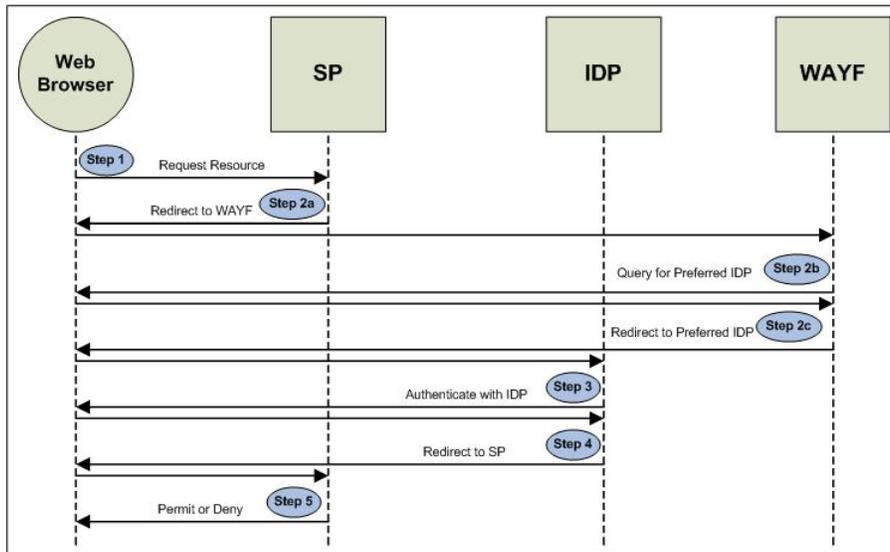
**Figure 10: Modified Shibboleth/SAML Web SSO Profile with a Where-Are-You-From (WAYF) Service**
