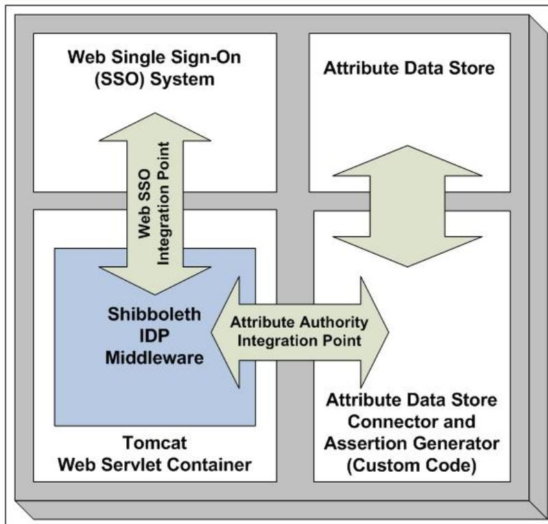
Figure 2: GFIPM Identity Provider (IDP) Structure
